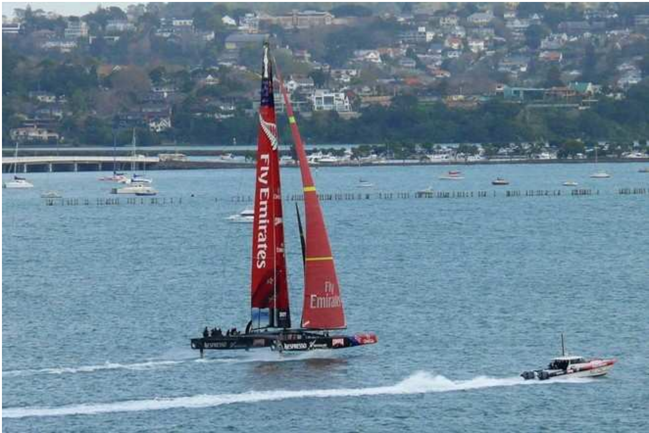
5 - AC72 - New Zealand fully lifted on her L-Foils and sailing on the Waitemata Harbour, Auckland, New Zealand. The windward L-foil is shown clear of the water in compliance with AC racing rules. - Swan Images Click Here to view large photo
